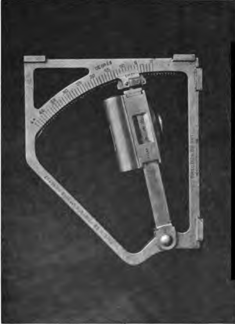
STANDARD GUNNER'S QUADRANT USED WITH MEDIUM AND HEAVY GUNS.
